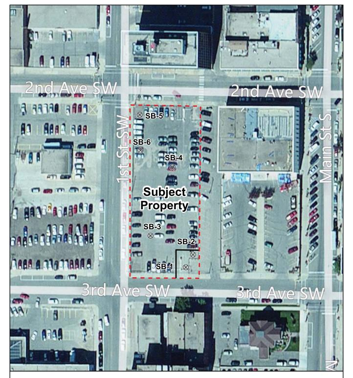
**Figure 2: Soil Boring Locations**
